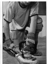
**SPECIFICATIONS DWE46100** DWE46101 DWE46151 Max Wheel Diameter 5" / 6' 5" / 6" 5" Hose Port Inner Diameter 35 mm 35 mm 35 mm Hose Port Outer Diameter 42 mm 42 mm 42 mm Tool Free Shroud Change Yes Yes Yes Tool Free Accessory Change Yes Yes Includes Universal connector, DWE46102 grinder Universal Connector and with quard, side handle, matched flange D28112 Grinder set, wrench and diamond blade
